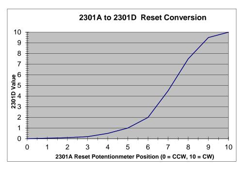
Figure B-2. Reset Potentiometer Conversion Chart
