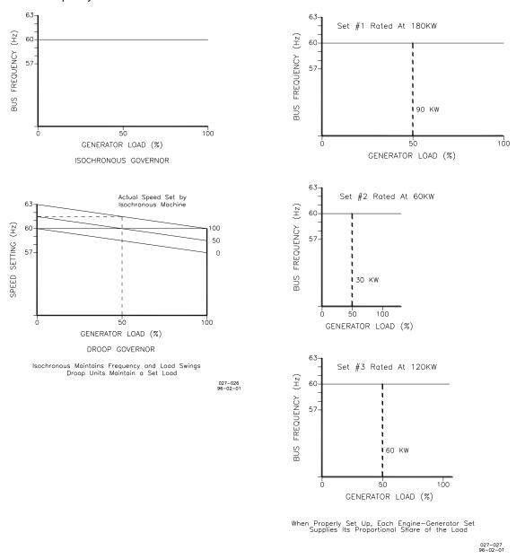
Figure 3-7. Droop/Isochronous Load Sharing
