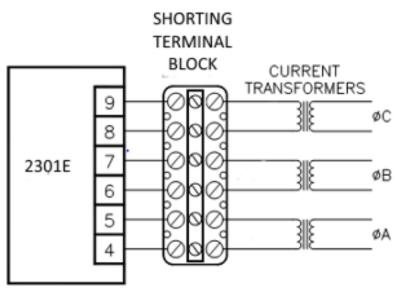
Figure 5-1. Temporary Wiring for Transformer Phase Correction
