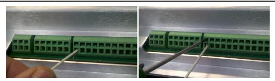
Figure 2-1. Installation of Wiring into Terminal
