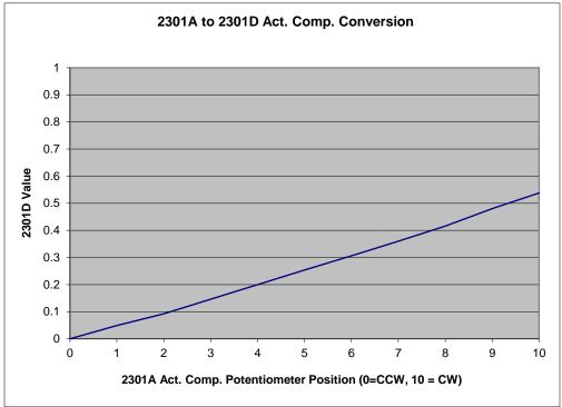
Figure B-3. Actuator Compensation Potentiometer Conversion Chart
