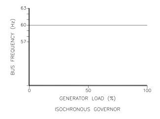
Figure 3-6. Isochronous Mode
