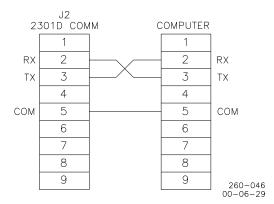
Figure 4-1. Null Modem Cable
