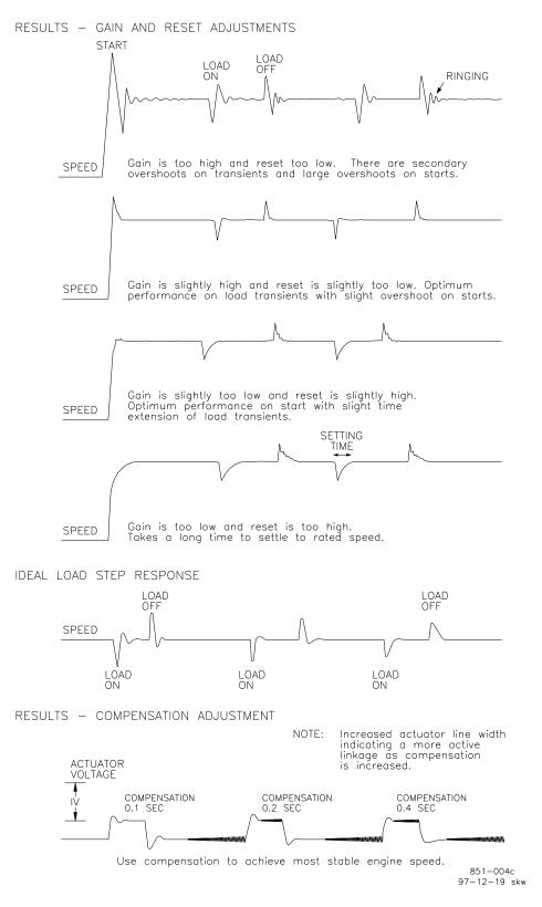
Figure 4-5. Typical Transient Response Curves
