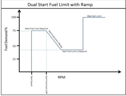
Figure 3-3. Dual Start Limit Function
