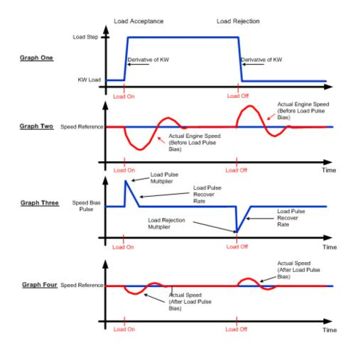
Figure 3-9. Load Pulse / Rejection
