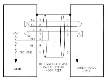
Figure 2-4. Typical RS-422 Communications Connections
