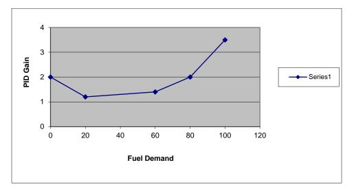
Figure 4-8. Linearized Gain Plot
