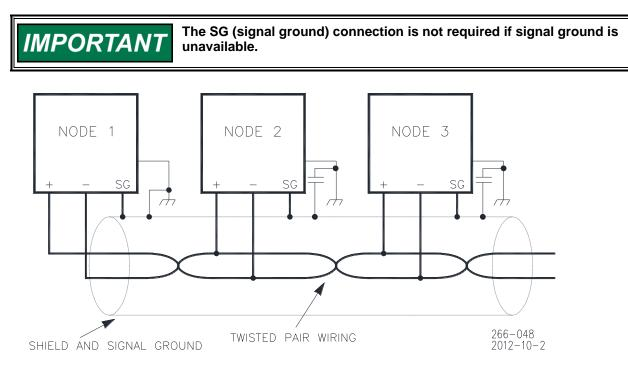
Figure 2-7. Alternate Multipoint Wiring Using Shielded Twisted-pair Cable without a Separate Signal Ground Wire
