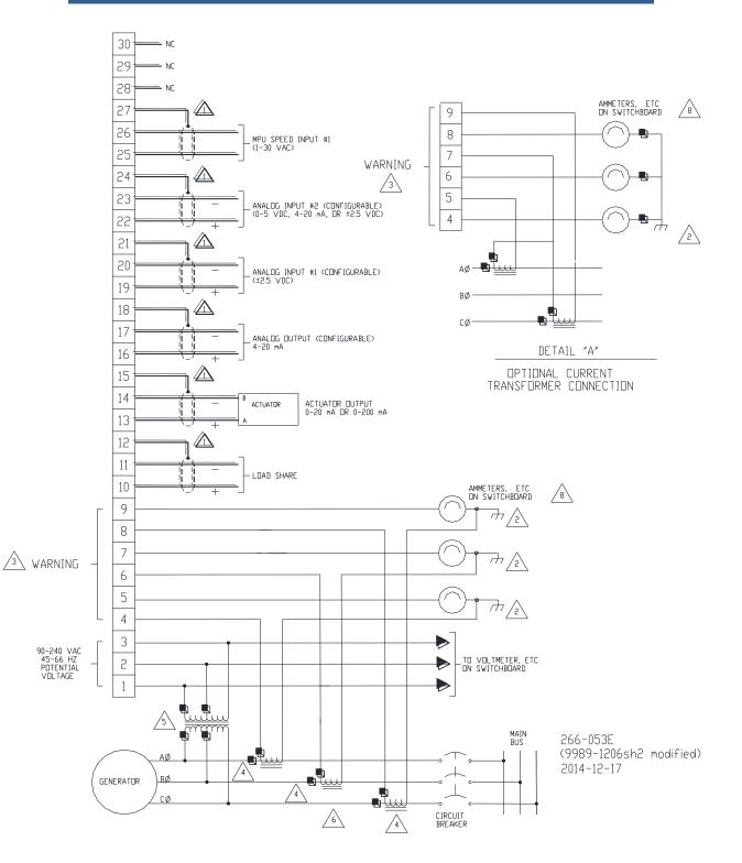
Figure 1-2a. 2301E Control Wiring Diagram (sheet 1)
