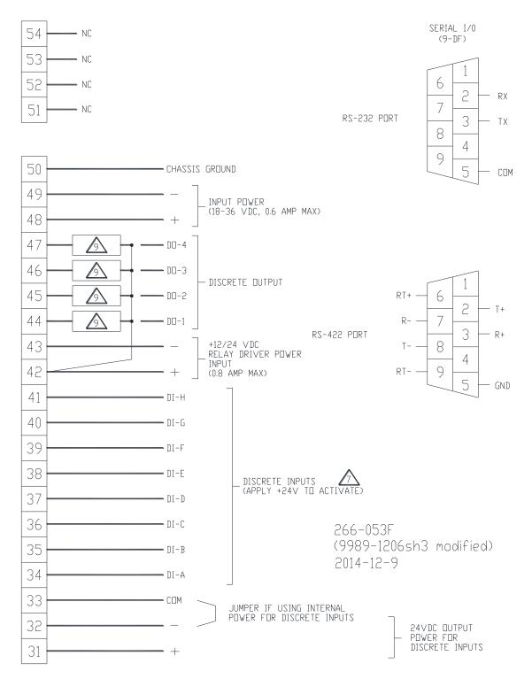
Figure 1-2b. 2301E Control Wiring Diagram (sheet 2)
