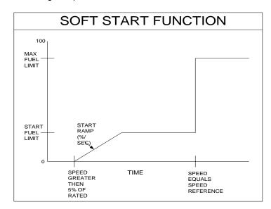
Figure 4-10. Soft Start Fuel Limit Function
