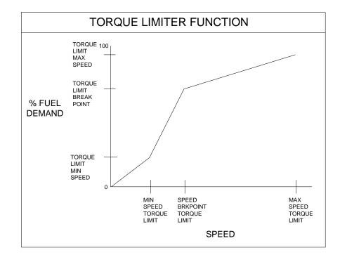
Figure 4-11. Torque Limiter Function
