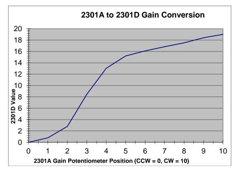
Figure B-1. Gain Potentiometer Conversion Chart
