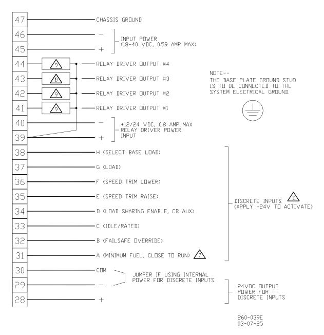
Figure 1-2. 2301D Plant Wiring Diagram (sheet 2)
