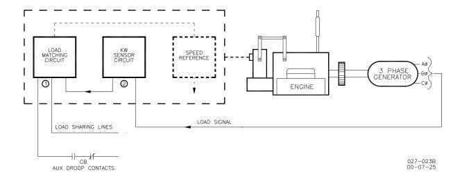
Figure 4-4. Paralleling System
