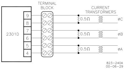
Figure 3-8. Temporary Wiring for Transformer Phase Correction
