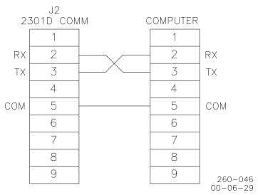
The drawing above shows the required connections in the null modem cable. These are the minimum connections, some purchased null modem cables have more interconnects, which are not used by the control.
