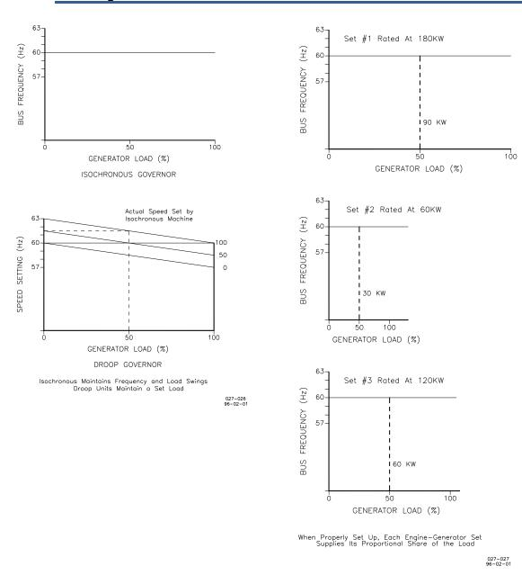
Figure 4-7. Droop/Isochronous Load Sharing
