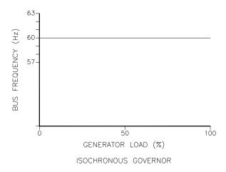
Figure 4-6. Isochronous Mode
