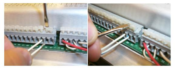
Figure 2-1. Installation of Wiring into Terminal
