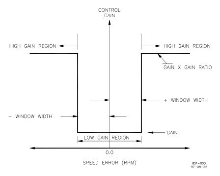
Figure 3-1. Control Gain as a Function of Speed Error
