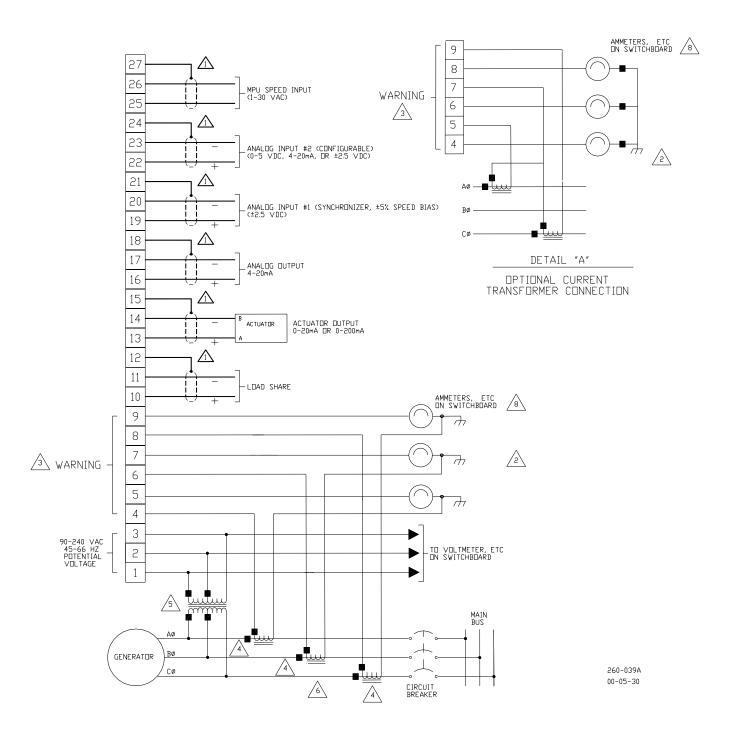
Figure 1-2. 2301D Plant Wiring Diagram (sheet 1)
