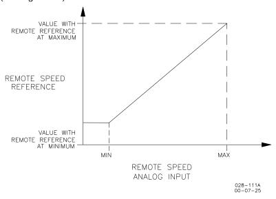
Figure 4-3. Remote Speed Reference
