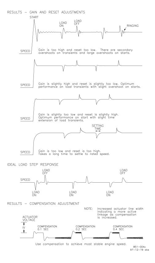
Figure 3-3. Typical Transient Response Curves
