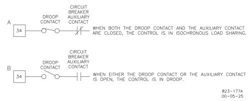
Figure 2-2. Droop Contact and Circuit Breaker Auxiliary Contact
