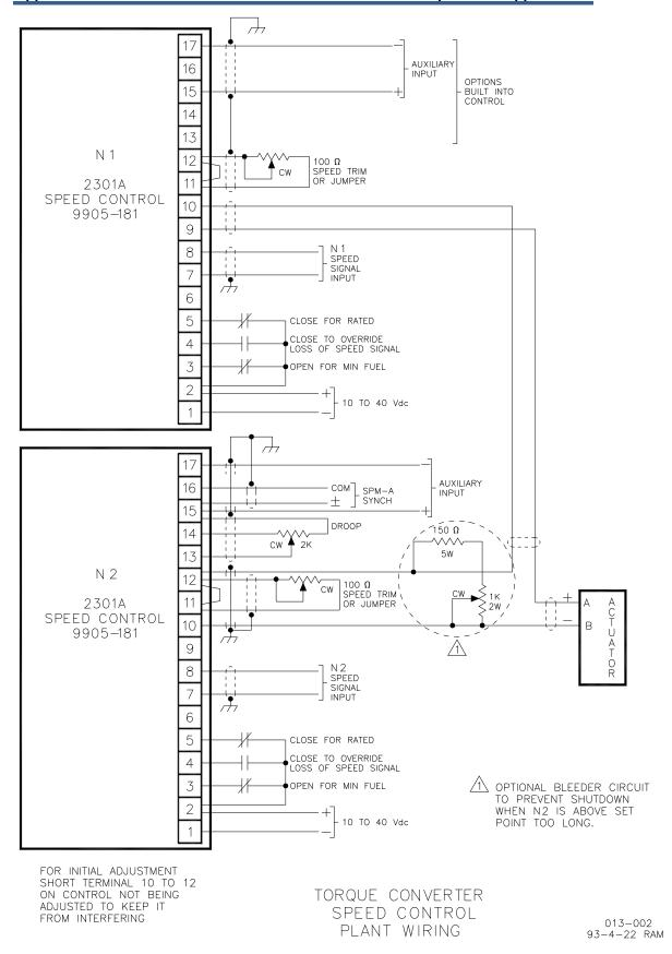
Figure 2-3. Plant Wiring Diagram, Split Shaft Speed Control
