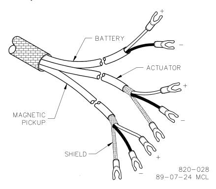
Figure 2-2. Preparation of Shielded Cables
