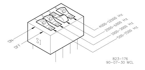
Figure 2-1. Speed Range Switch
