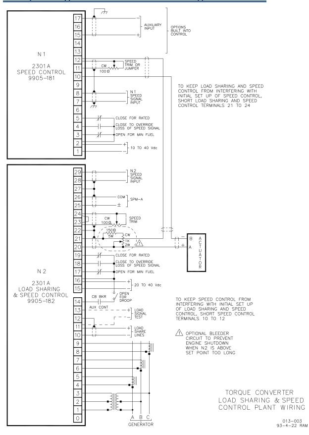
Figure 2-4. Plant Wiring Diagram, Split Shaft Load Sharing and Speed Control
