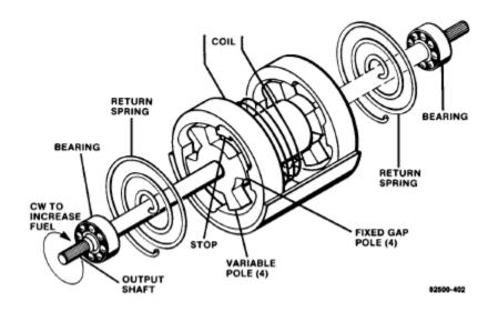
Figure 4-2. Actuator Schematic
