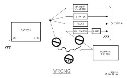
Figure 2-6. Correct and Incorrect Wiring to Battery
