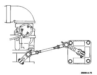
Figure 2-4. Carburetor Compensating Linkage at Maximum Fuel
