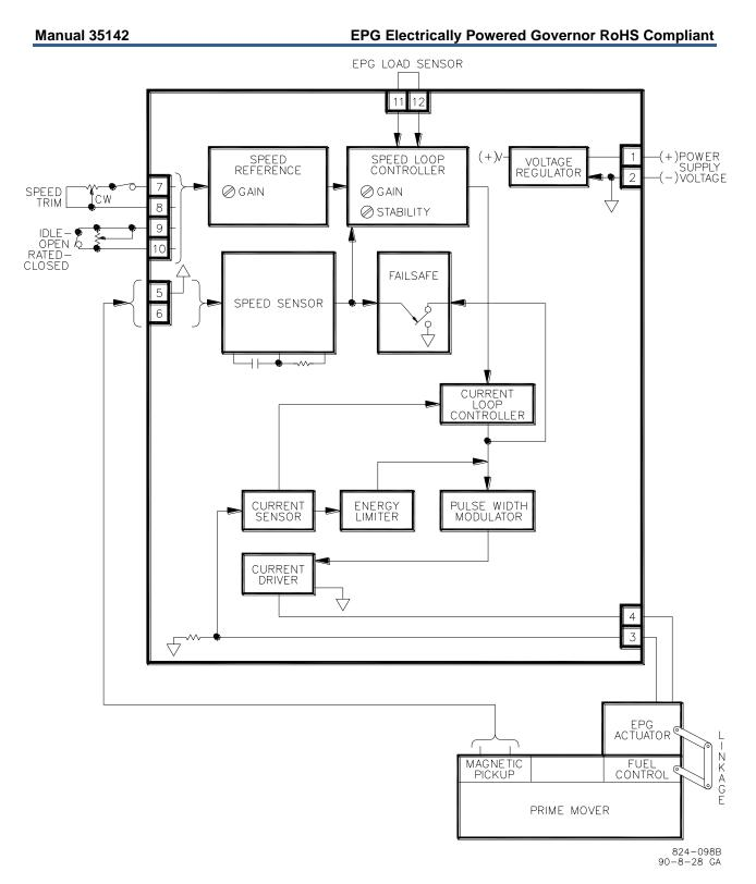
Figure 4-1. EPG Block Schematic Diagram
