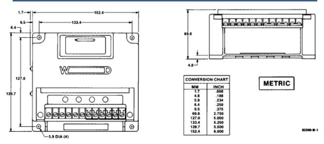
Figure 1-2. Outline Drawing for EPG 512/1712 and 524/1724 Speed Controls (Do not use for construction.)
