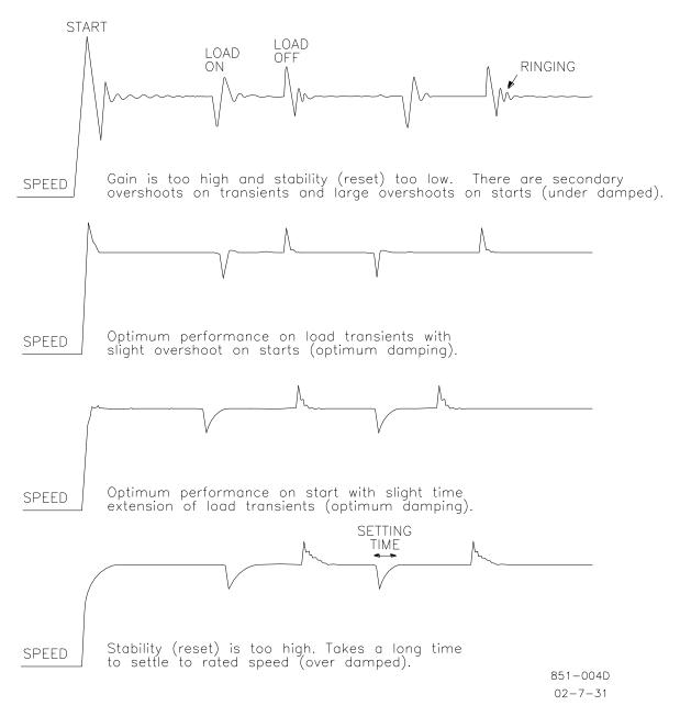
Figure 2-7. Starting and Transient Response Curves
