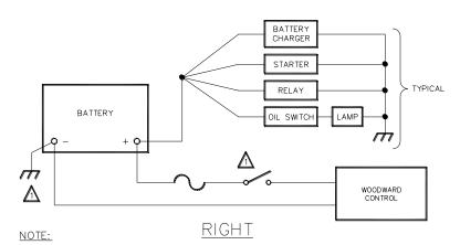
$\Lambda$  a negative ground system is shown. If a positive ground system is used, the switch and fuse must be located in series with battery (-) and terminal (Tb1-2) on the woodward control. The positive terminal becomes chassis ground.
