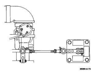
Figure 2-3. Carburetor Compensating Linkage at Minimum Fuel
