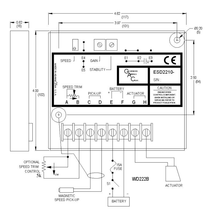
See specific actuator publication for proper wiring of actuator connector for battery voltage used.
