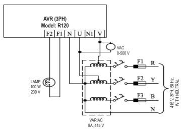
STATIC TEST CONNECTION DIAGRAM OF 3PH AVR
