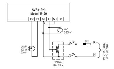
STATIC TEST CONNECTION DIAGRAM OF 1PH AVR
